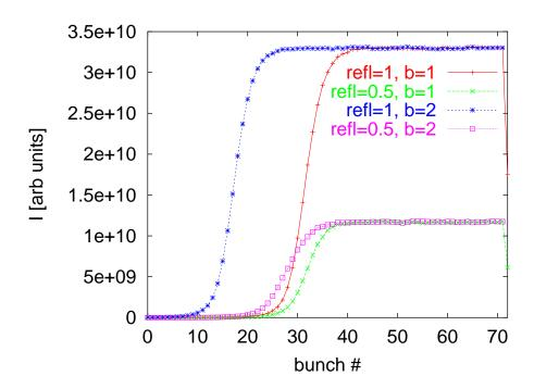
SPS measurement consistent with 50% or 100% dedicated experiment to measure decay can contrain reflection
