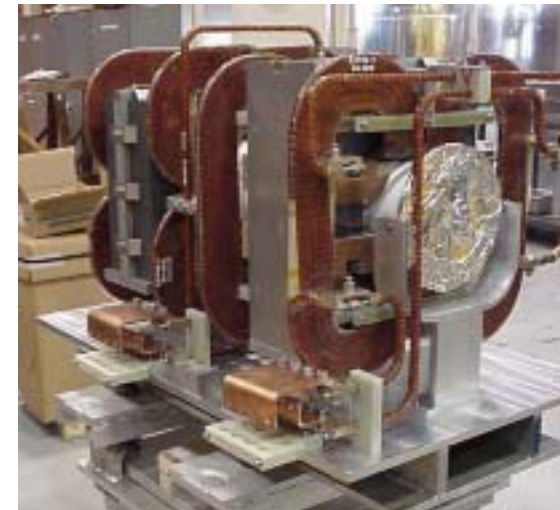
Short kickers w/ common ceramic chamber
