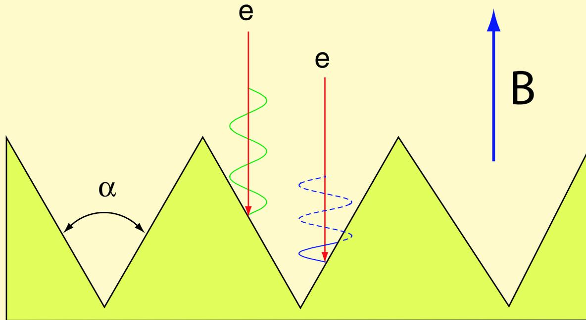
For 200 eV electron, the Larmor radius  $r_L$  in 1 Tesla field is about 25 microns. In the limit when  $r_L \ll$  size of grooves, the effective SEY does not depend on  $r_L$  and is only a function of  $\alpha$ .
