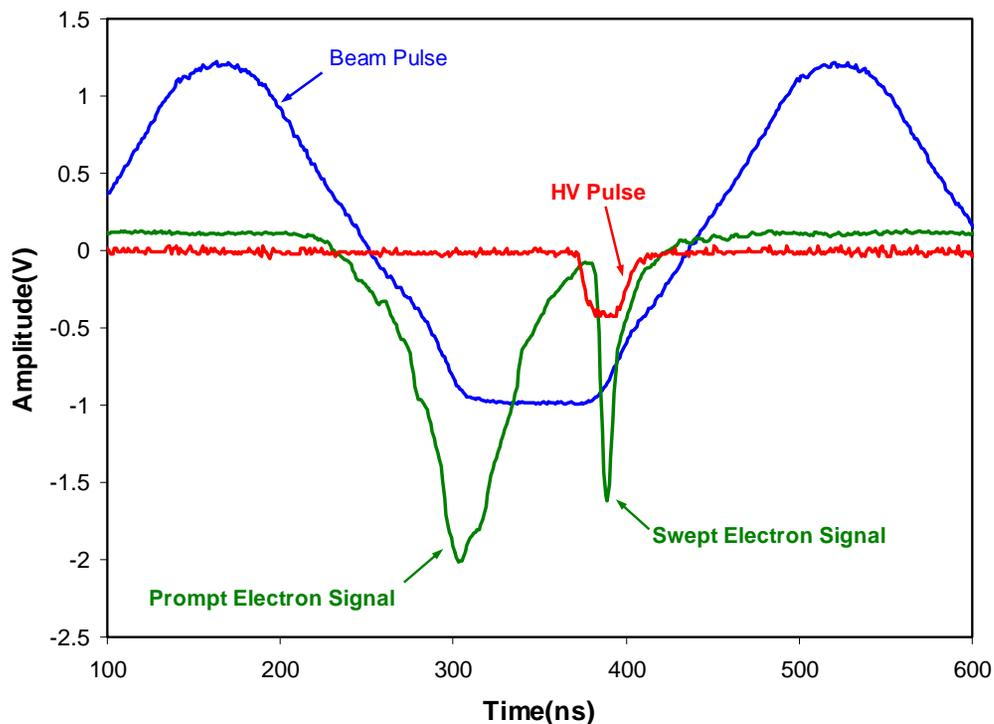
7.7  $\mu\text{C}$ /pulse, bunch length = 280 ns, 30 ns injection notch, signals averaged for 32 macropulses, repeller = - 25V, HV pulse = 500V
